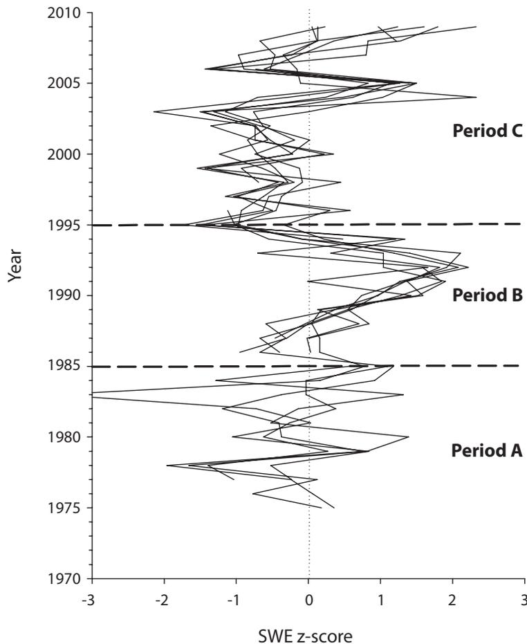
**Figure 6.** Z-scores of snow water equivalent (SWE) for snow courses in the Pelly Crossing region (see Table 2 for details about each snow course; Water Resources Branch, 2010b). Data from each snow course have been superimposed on this figure. The vertical dotted line represents a z-score of 0 and acts as a reference point, while the horizontal heavy-dashed lines indicate interpreted periods of decadal-scale shifts in SWE.
