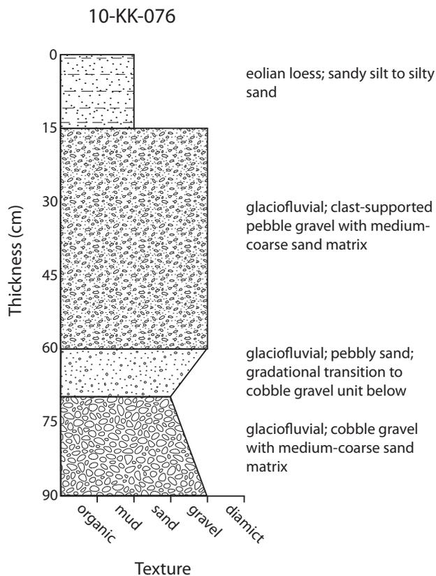
**Figure 18.** Measured stratigraphic section 10-KK-076; see Figure 1 for section location.
