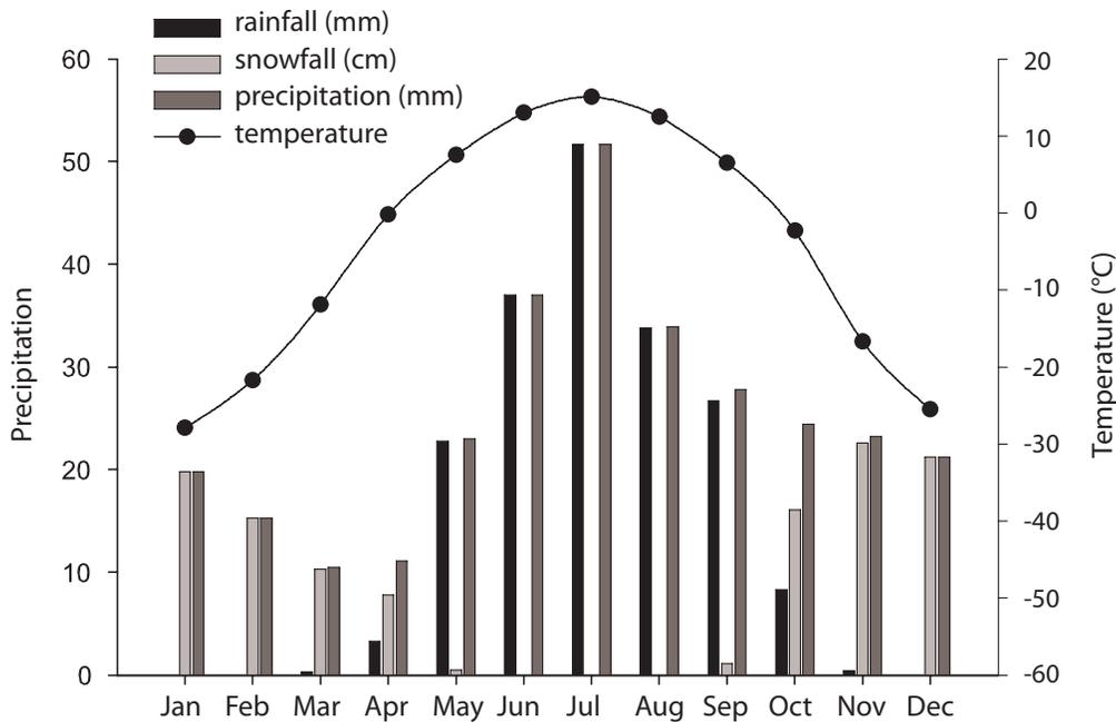
**Figure 2.** Climate normal (1961-1990) temperature and precipitation for the Pelly Ranch meteorological monitoring station (Environment Canada, 2010). To calculate total precipitation in millimetres, snowfall was converted to snow water equivalent (SWE) and summed with rainfall.
