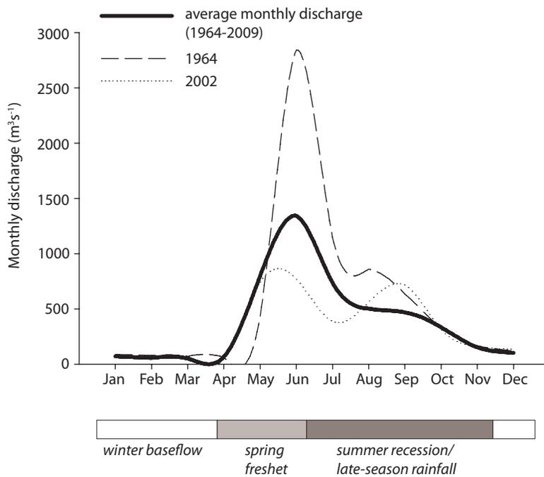
**Figure 4.** Hydrograph depicting average monthly discharge for the Pelly River at Pelly Crossing (heavy solid line). Also shown are hydrographs for the years 1964 (long-dashed line) and 2002 (dotted line), demonstrating high and low June discharge, respectively. The 2002 hydrograph also exhibits a secondary peak in late summer/autumn in response to late-season rainfall (Water Survey of Canada, 2010).
