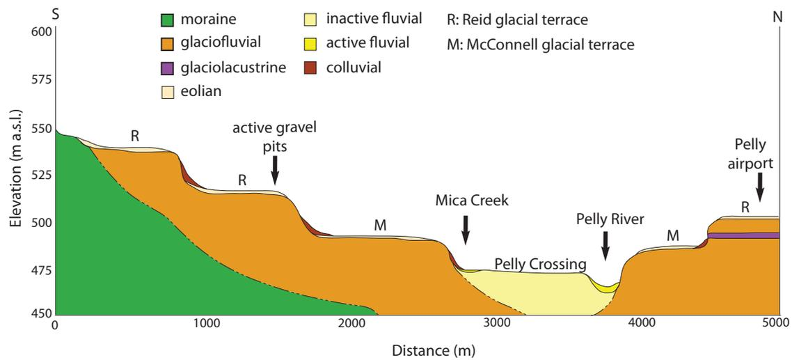
**Figure 15.** A profile of the distribution of surficial sediments in the Pelly Crossing area illustrates multiple levels of glaciofluvial terraces and probable subsurface contacts.
