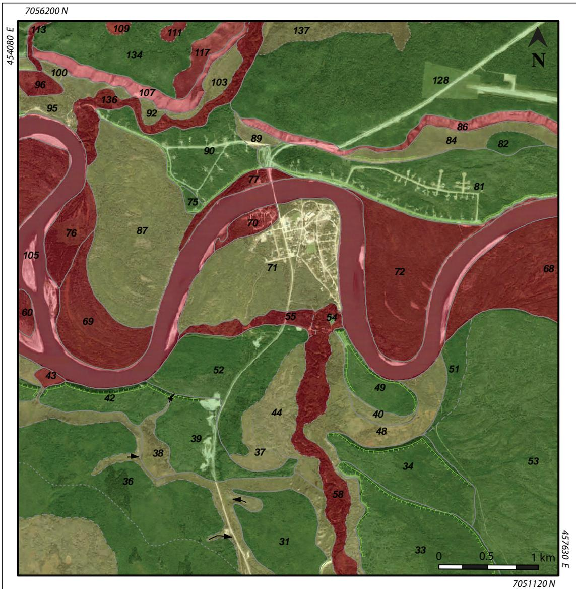
**Figure 23.** Detailed view of hazard rankings in the developed area surrounding the community of Pelly Crossing. Polygon numbers are discussed in the text and summarized in Appendix C. High, medium and low hazard rankings are represented by red, yellow and green polygons, respectively.
