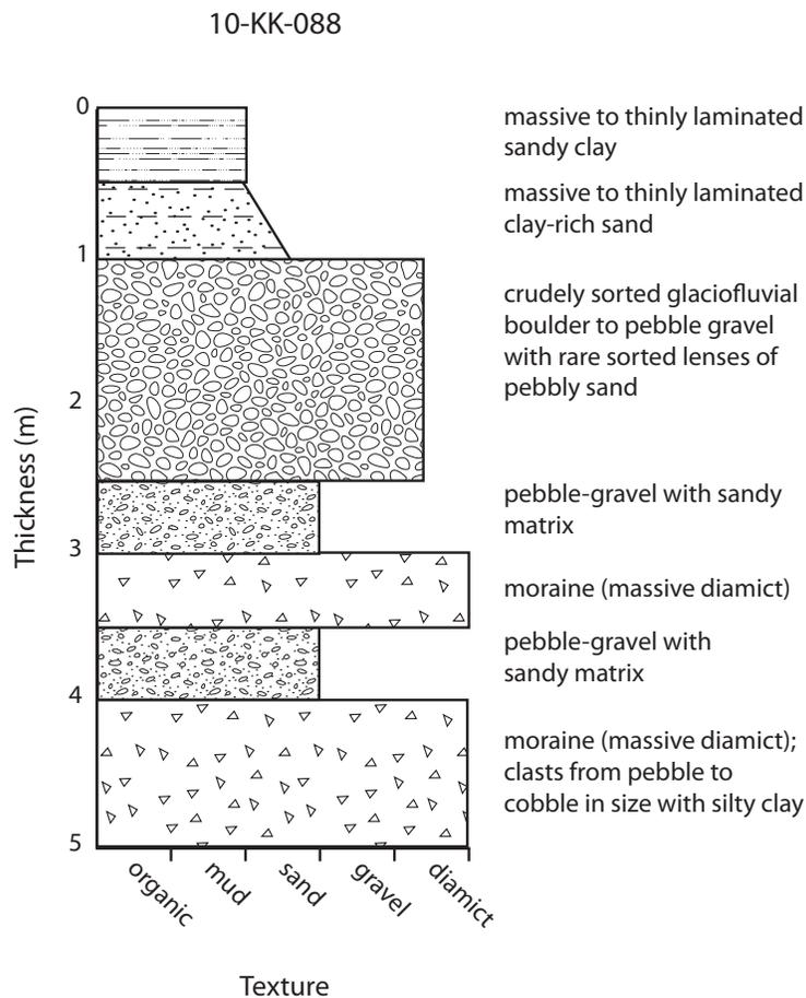
**Figure 16.** Measured stratigraphic section 10-KK-088; see Figure 1 for section location.
