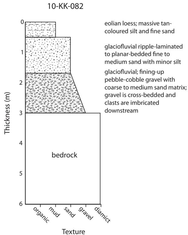
**Figure 20.** Measured stratigraphic section 10-KK-082; see Figure 1 for section location.
