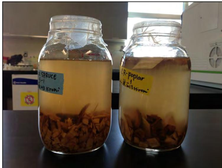
Figure 2 Carbon release batch test
