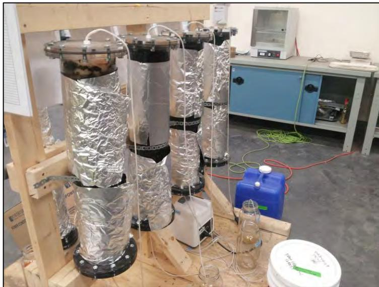
Figure 7 Bioreactors C5 to C8 (Wolverine conditions (Biopass), 14 cm ID)
