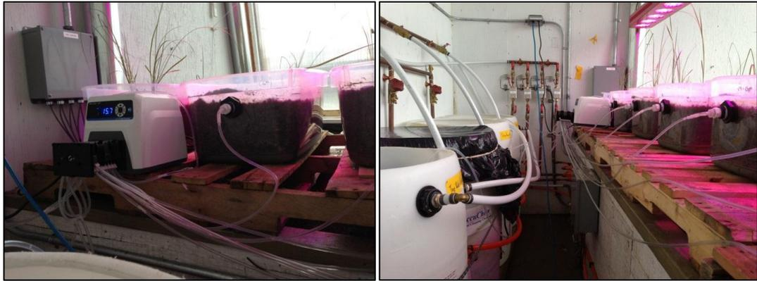
**Figure 5** Synthetic influents or tap water being pumped at the bottom of the substrate using a multi-channel peristaltic pump (Masterflex pump, head and C-flex tubing) at 5 ml/min with sub-surface vertical flow.
