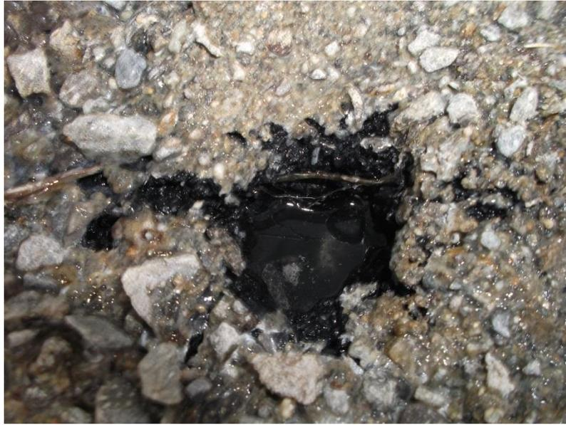
**Figure 9** Black deposits on the wetland surface, characteristic of sulfide precipitates found only in the Pit(MeOH) CW treatment. In addition, an odiferous evidence of H<sub>2</sub>S from the Pit(MeOH) was present.
