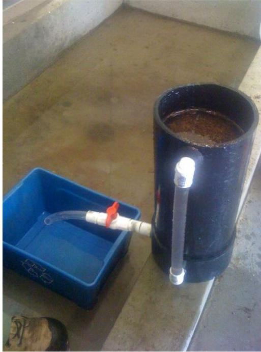
**Figure 4** Hydraulic conductivity testing to determine the appropriate ratio of peat, sand and pea gravel to achieve a 5 ml/min flow rate with a hydraulic residence time of approximately 5 days.
