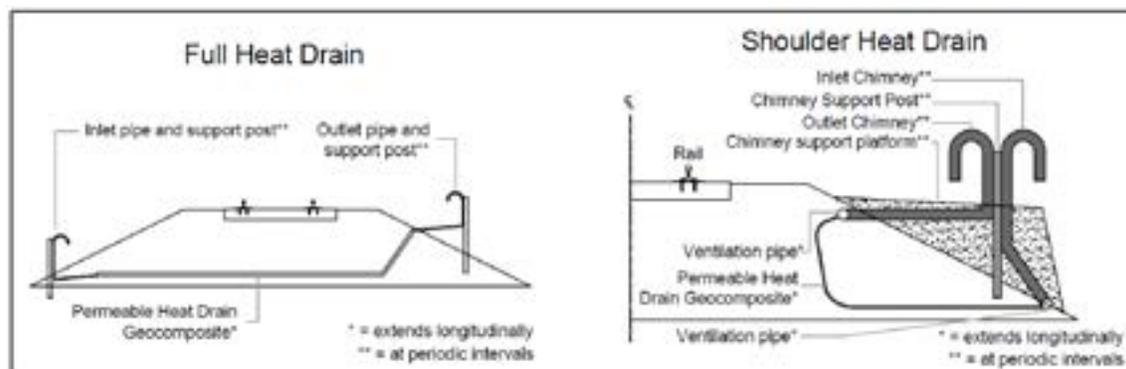
Figure 12. Heat drains (Regehr et al., 2012).
