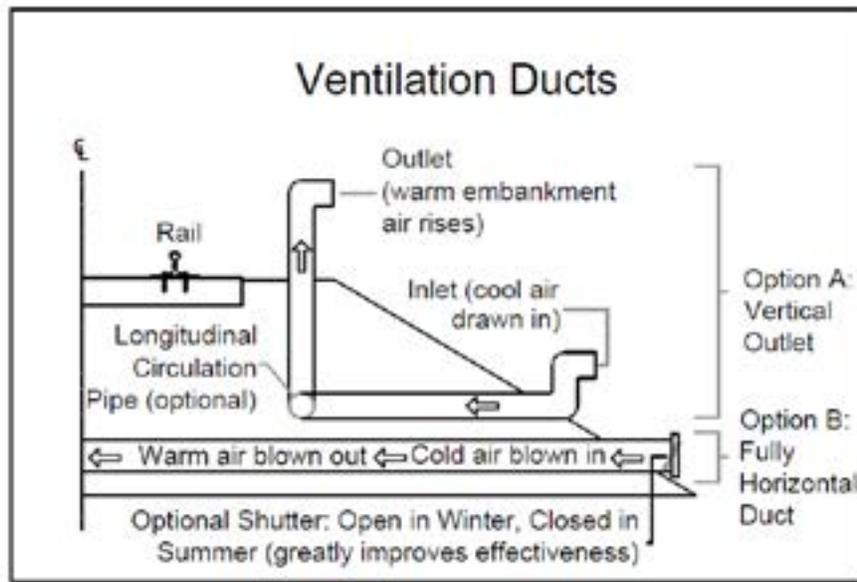
**Figure 10.** Ventilation duct design (Regehr et al., 2012).
