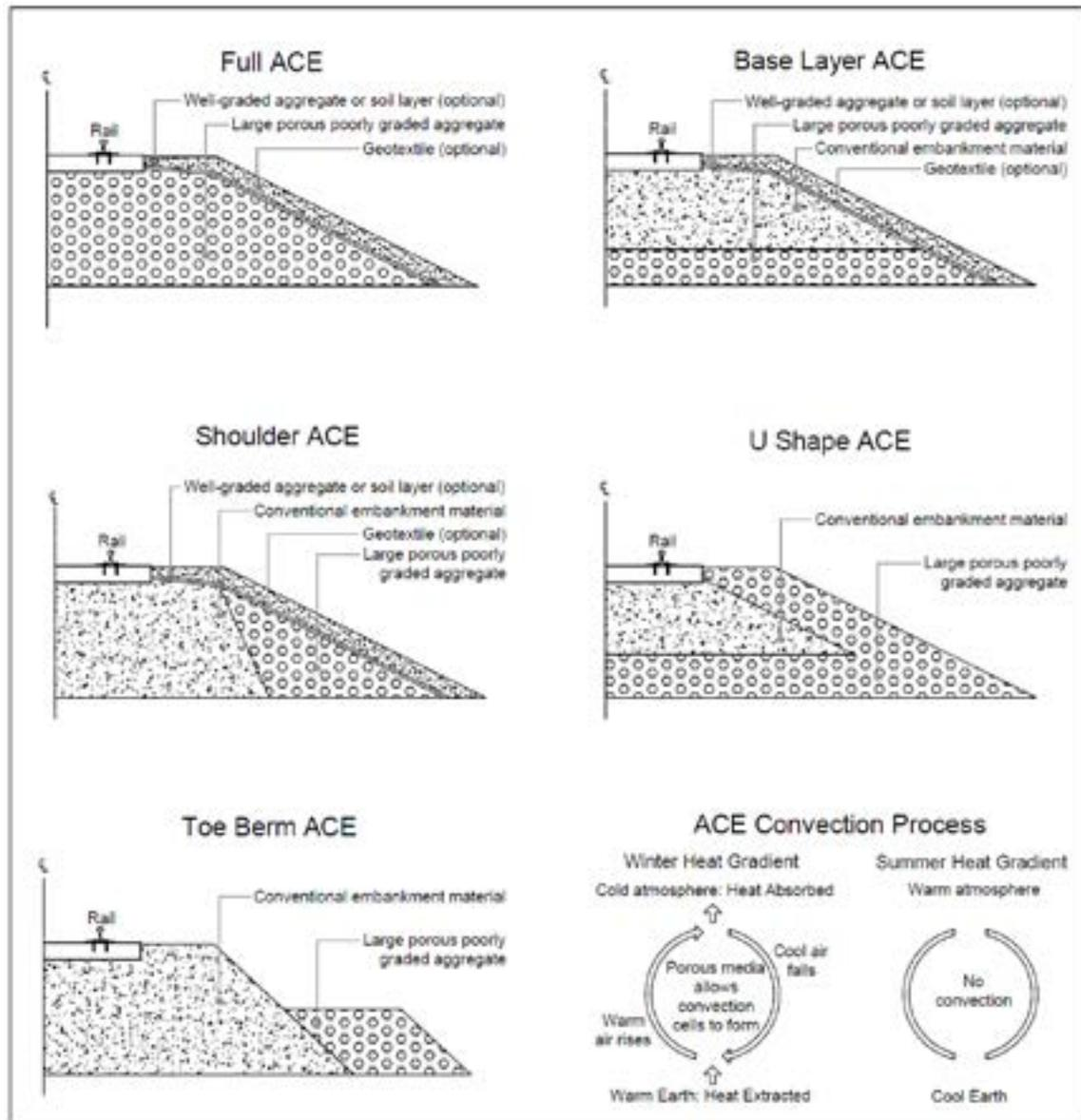
**Figure 9.** Variations on the air convection embankment (ACE) design configurations (Regehr et al., 2012).
