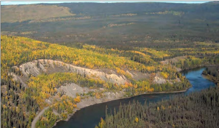
**Figure 21.** Rotational slump near km 9 of the North Canal Road (station 13DT37). Road construction and river erosion are undercutting the toe of the slide and contributing to instability. The slump is approximately 70 m tall, 250 m wide, and 180 m long.
