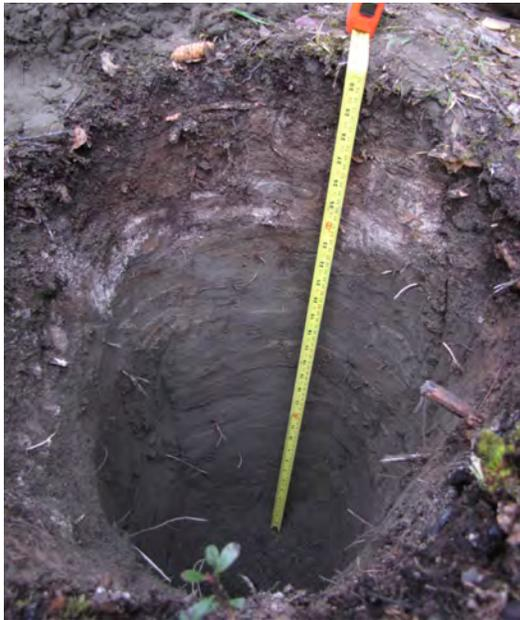
**Figure 39 (left).** Fine-grained fluvial sediments exposed in an 80 cm-deep soil pit dug at the Kulan Street site (station 13DT046). Pockets of White River ash are visible just below the brown surface organic layer.
