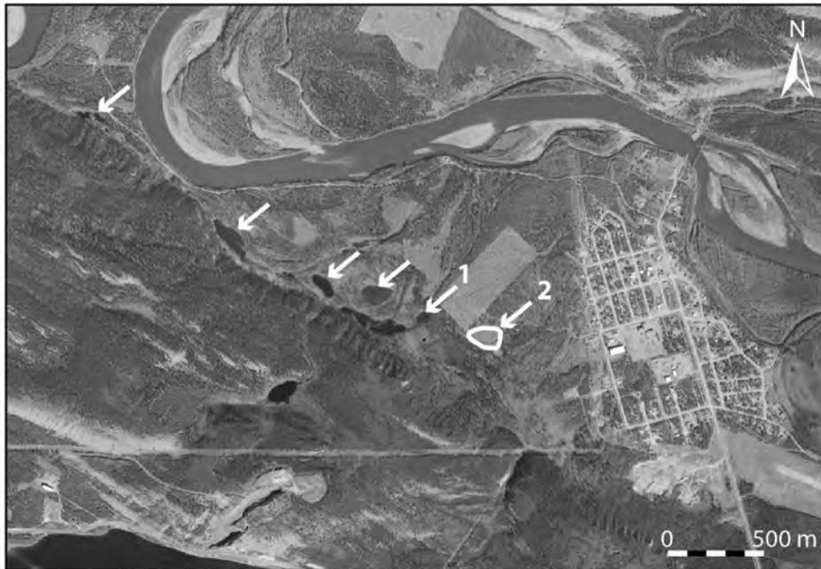
**Figure 23.** Thermokarst collapse ponds visible on a 2007 air photograph (National Air Photo Library A28547-233) are highlighted by white arrows. Comparison with historical air photographs shows that at a new pond has developed since 1967 (see point 1), while an old pond that was present in 1967 has since filled in with organic materials (see point 2).
