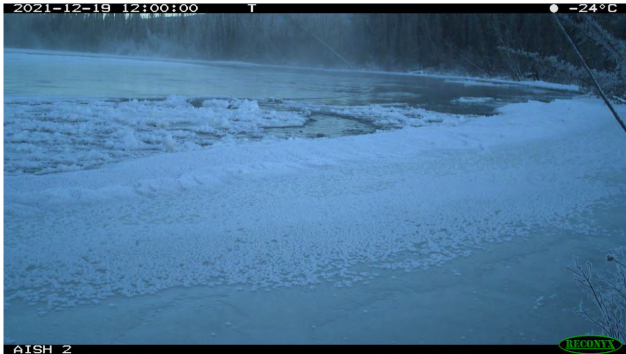
Figure 4.2.4. Frontal progression of a mid-channel frazil jam at Kp 12 of the Āshèyi Chu (looking upstream).
