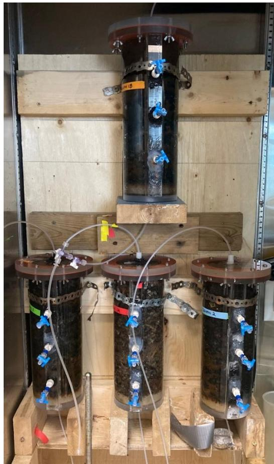
Figure 5. The columns were maintained at 5°C for the duration of the experiment. Note C1 in the centre, comprised of two columns in series.
