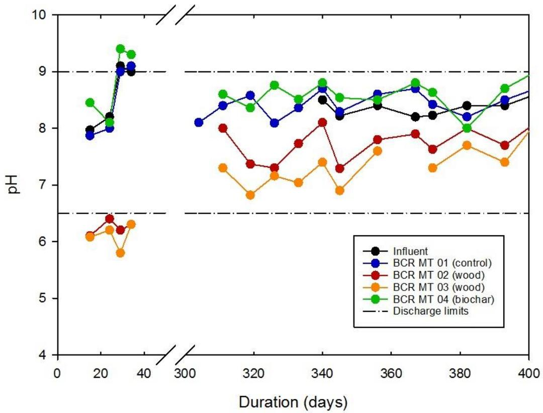
**Figure 7.** pH in influent and effluent of the four bioreactors (BCR-MT-01 to -04) between August 20<sup>th</sup> 2014 to September 26<sup>th</sup> 2015 (Discharge Limit Range: 6.5 to 9).
