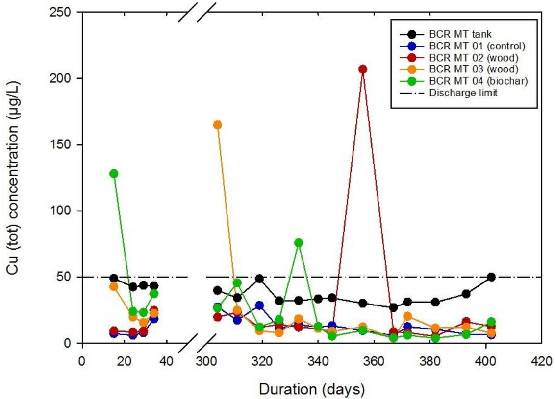
**Figure 2.** Copper concentrations in influent and effluent of the four bioreactors (BCR-MT-01 to -04) between August 20<sup>th</sup> 2014 and September 26<sup>th</sup> 2015 (Discharge Limit of 0.050 mg/L).
