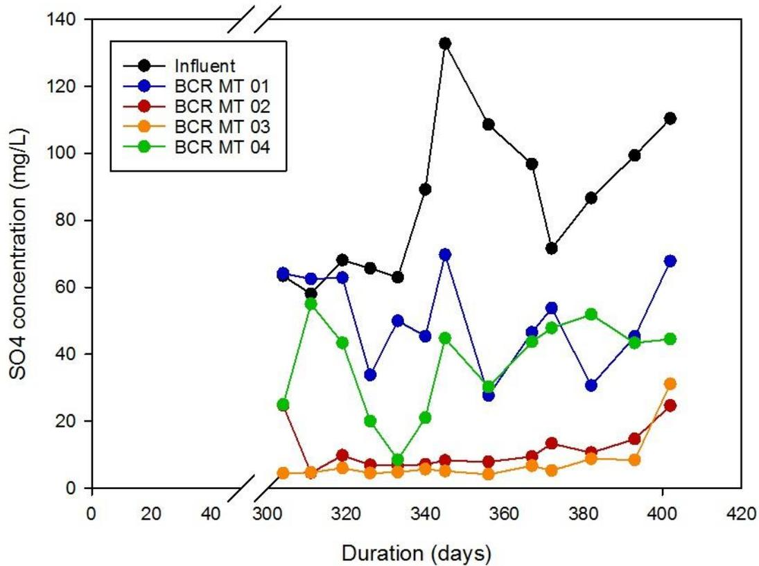
**Figure 30.** Total Sulfate in influent and effluent from the four bioreactors (BCR-MT-01 to -04) between August 20<sup>th</sup> 2014 to September 26<sup>th</sup> 2015.
