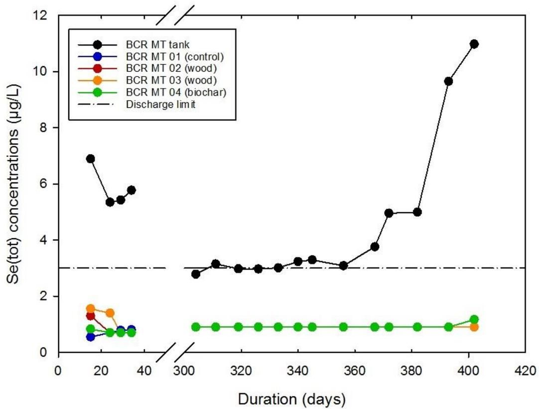
**Figure 5.** Selenium concentration in influent and effluent of the four bioreactors (BCR-MT-01 to -04) between August 20<sup>th</sup> 2014 and September 26<sup>th</sup> 2015 (Discharge Limit of 0.003 mg/L).
