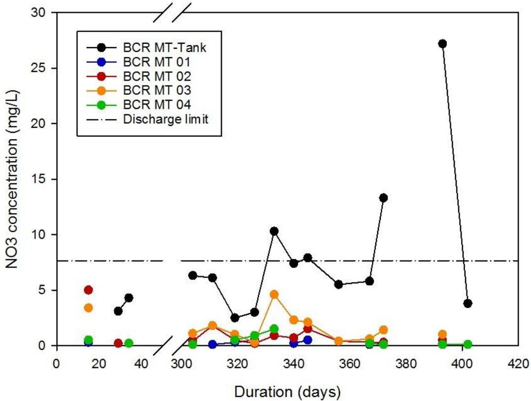
**Figure 8.** NO<sub>3</sub> concentrations in influent and effluent of the four bioreactors (BCR-MT-01 to -04) between August 20<sup>th</sup> 2014 and September 26<sup>th</sup> 2015 (Discharge Limit of 7.65).
