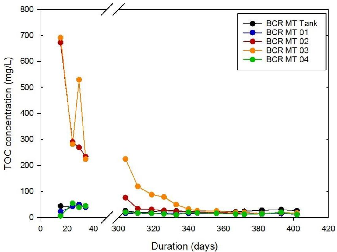
**Figure 9.** Total Organic Carbon in influent and effluent from the four bioreactors (BCR-MT-01 to -04) between August 20<sup>th</sup> 2014 and September 26<sup>th</sup> 2015.
