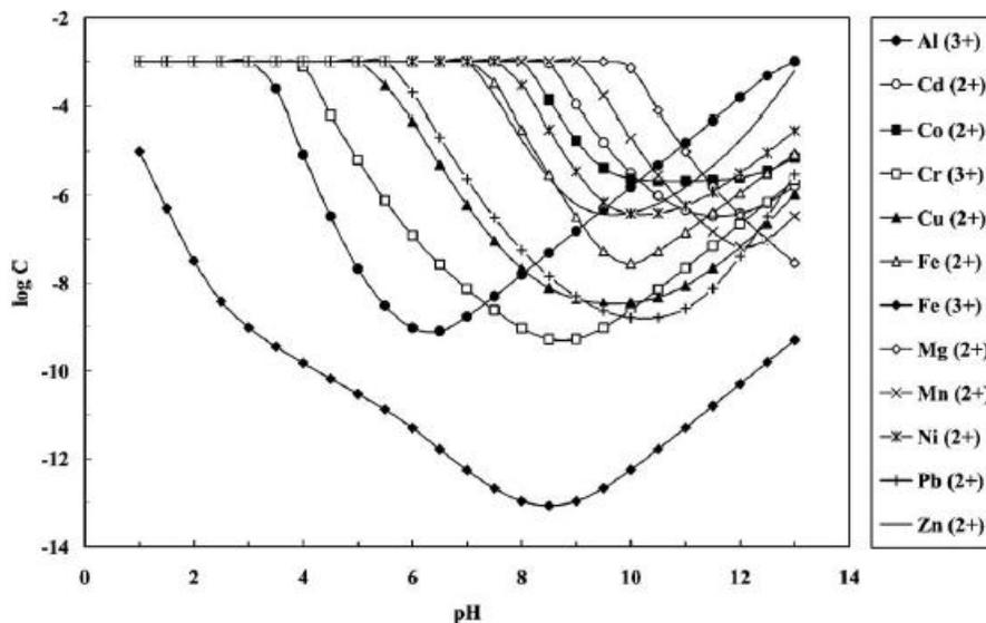
**Figure 5: Solubility of different metal hydroxides based on chemical equilibrium calculations using the MINQL+ software. Stimulation conditions: T=25°C, Cl<sub>i</sub>=10<sup>-2</sup> M and (metal)<sub>i</sub> = 10<sup>-3</sup>M (Blais et al, 2008, p.137).**
