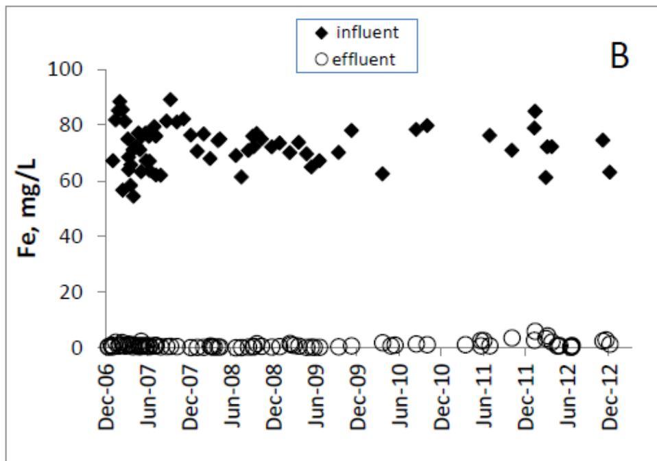
**Figure 20: Total Fe concentration at influent and effluent of the Marchand mine treatment system, Pennsylvania (Hedin, 2013, p.10).**
