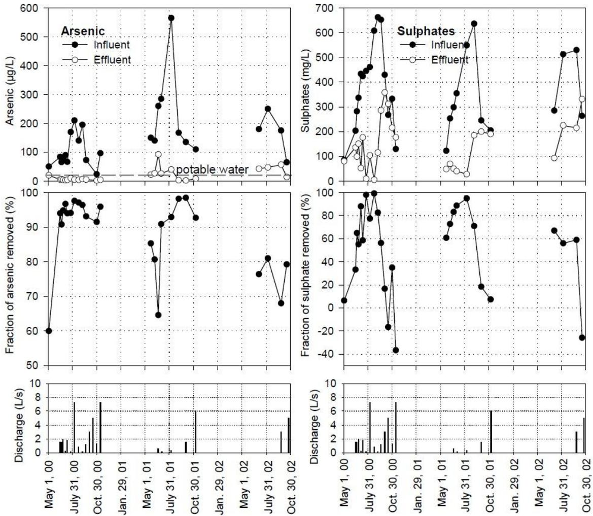
**Figure 22: Arsenic and sulphates at the influent and effluent of the biofilter and their respective fraction removed from May 2000 to October 2002. Measured discharge rates are also shown (Germain and Cyr, 2003, p. 7).**
