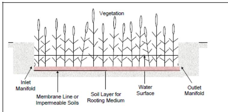
Figure 2a: Surface flow wetland (adapted from a drawing by SC Reed from EPA, 2000a, p. 1).
