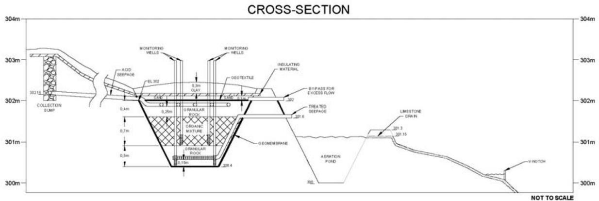
**Figure 17: Bioreactor design at the Cadillac mine in Quebec (Kuyucak et al, 2006, p. 988).**
