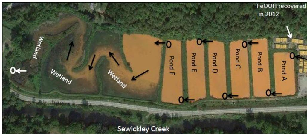
**Figure 19: Aerial view of the Marchand mine bioreactor ponds, wetlands and recovered iron sludge (Hedin, 2013, p.9).**
