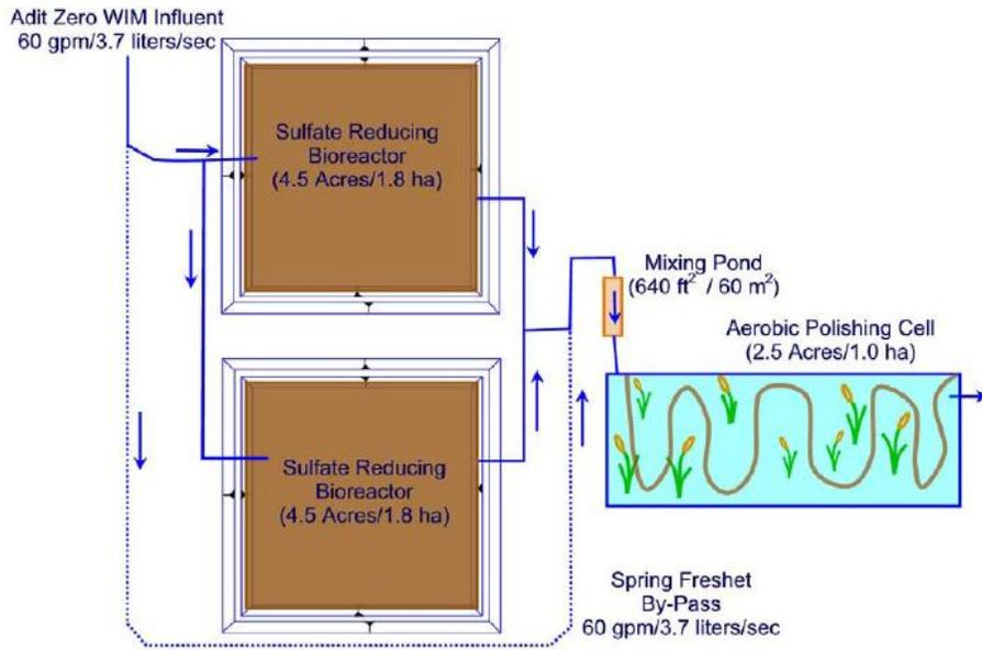
**Figure 4: Hypothetical hybrid system with bioreactor and aerobic wetland components (Gusek & Conroy, 2007, p. 265).**
