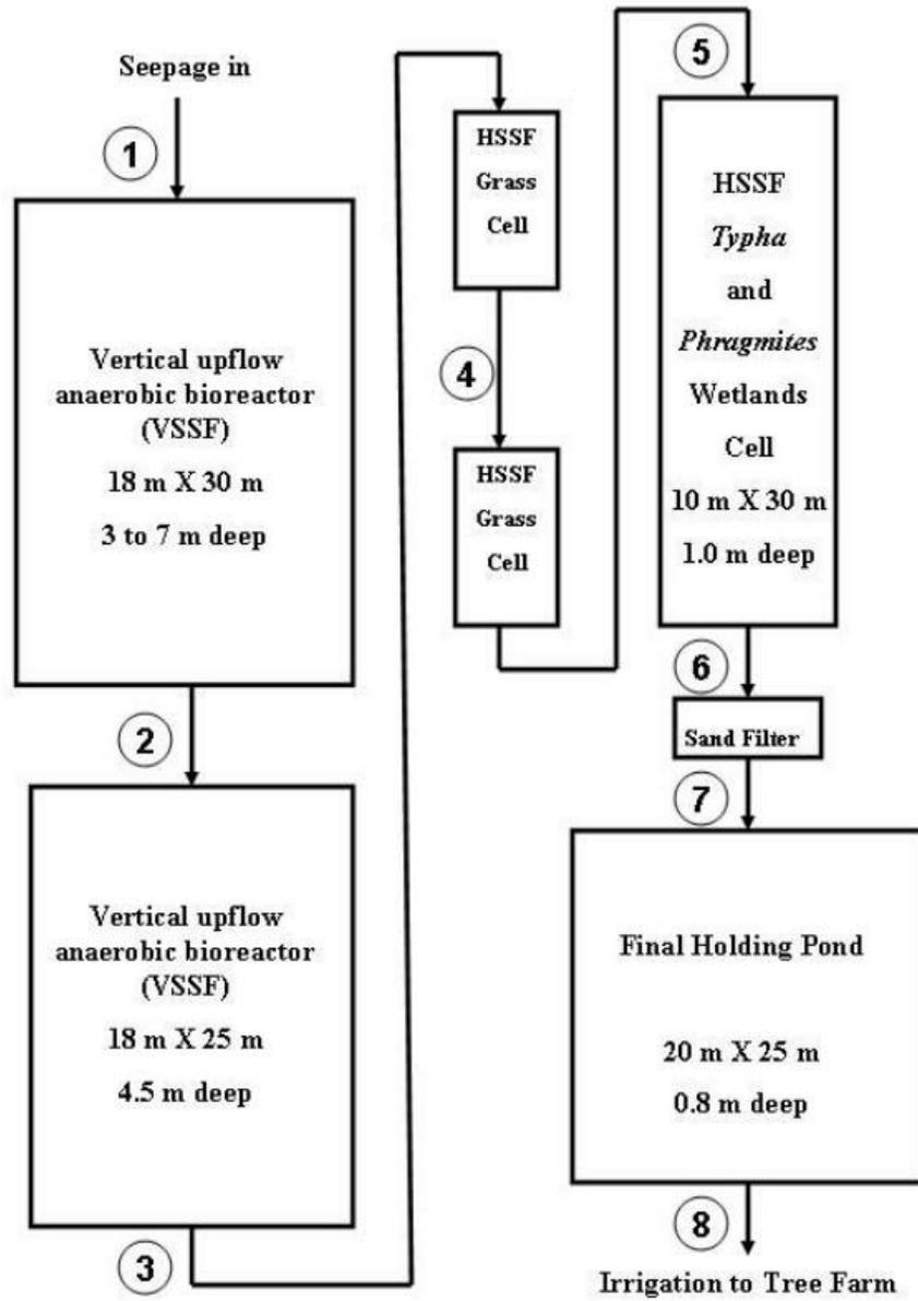
Figure 21: Diagram of the sequence of PT components at the Teck smelter, Trail, BC (Duncan, 2010, p. 40).
