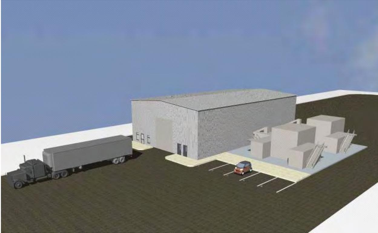
Option #3 retains the technical and operational characteristics of Option #1, but attempts to reduce costs by only enclosing the fuel handling area. This option would only be available for the CPC and Proton Power units as they are self-contained in standard shipping containers (CPC units depicted in the rendering).
