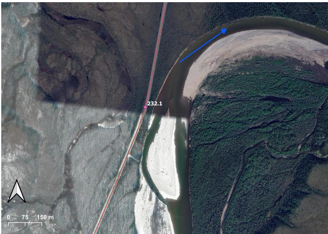
Figure 10. KM 232.1 of Dempster Highway. Separation distance = 23 m, risk rating = High, imagery date (top half): June 7, 2023.
