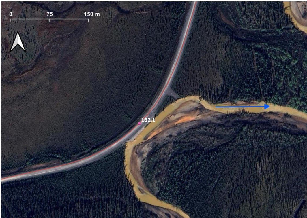
Figure 5. KM 182.1 of Dempster Highway. Separation distance = 0 m, risk rating = Very High, imagery date: June 4, 2023.
