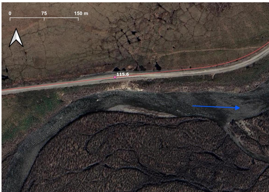
Figure 1. KM 115.6 of Dempster Highway. Separation distance = 9 m, risk rating = Very High, imagery date: June 2, 2023.
