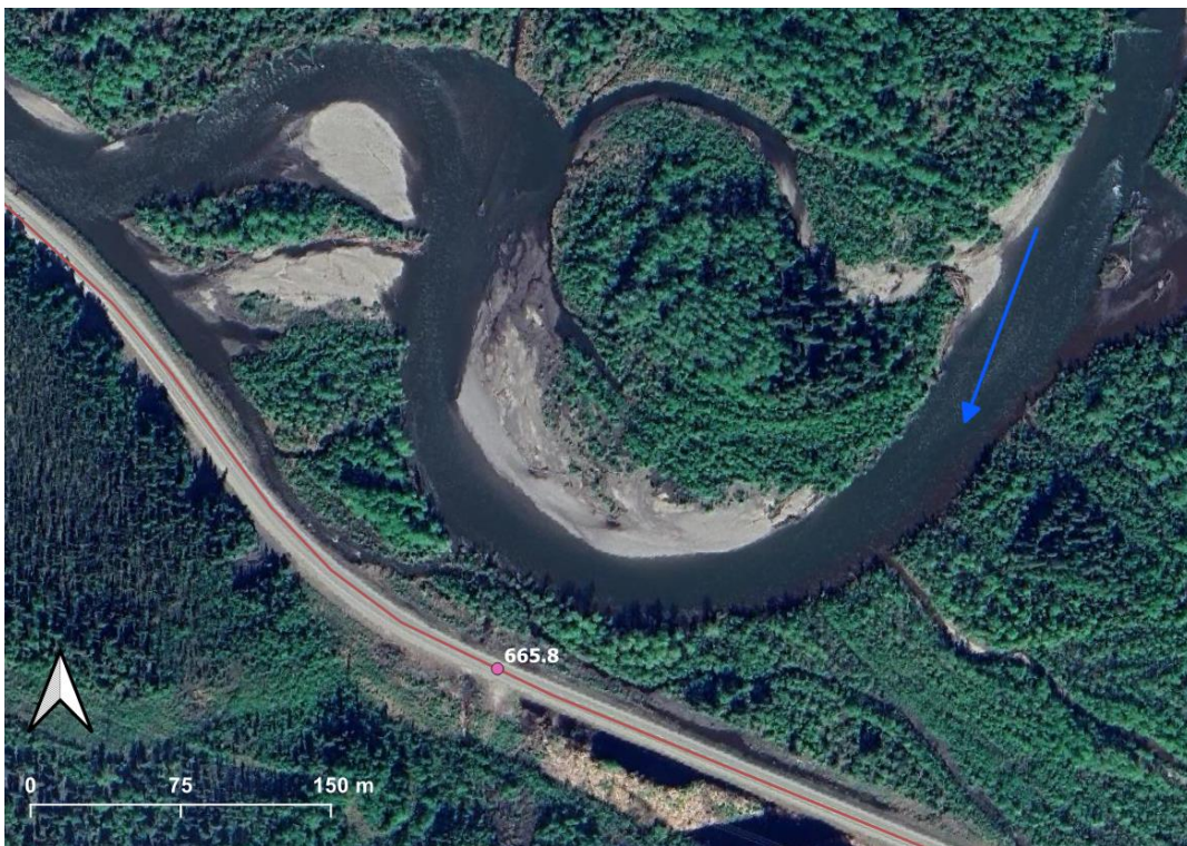
Figure 12. KM 665.8 of Klondike Highway. Separation distance = 34 m, risk rating = Moderate, imagery date: June 4, 2023.
