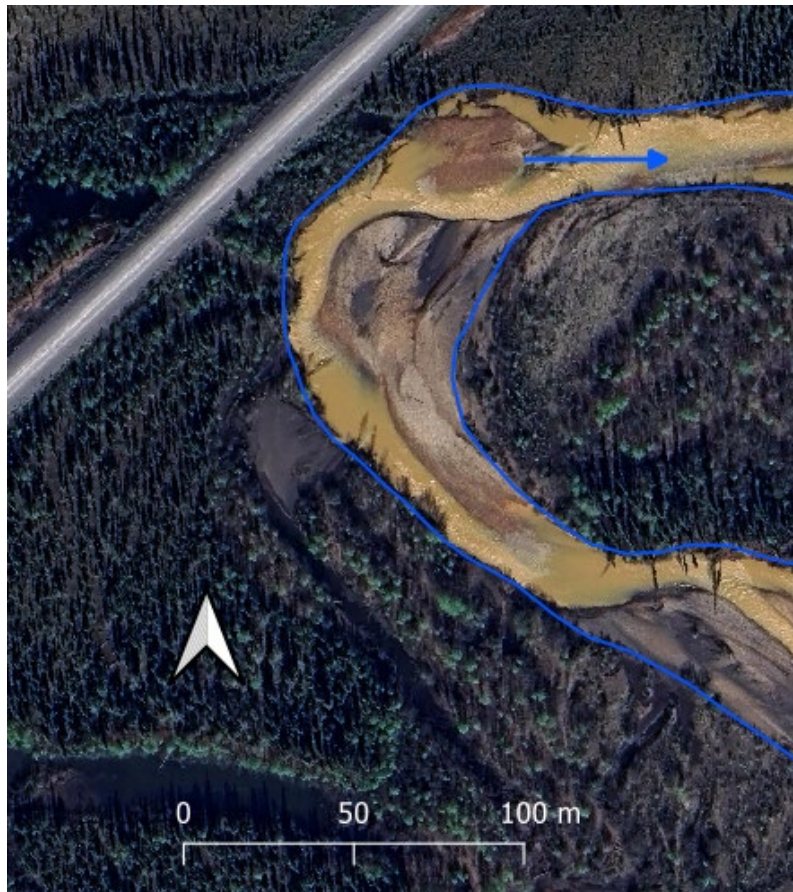
FIGURE 4.2. EXAMPLE OF TOP OF BANK DELINEATION (2023) AT DEMPSTER HIGHWAY KM 183.3.
