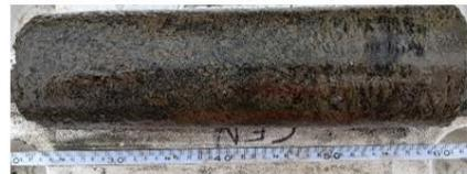
**Figure 28** A) The Inukjuak airport around 2018. Note the drainage ditches with standing water on both sides. Ice-rich permafrost cores recovered during the geotechnical investigation done in summer 2021 (L'Hérault et al., in prep.); B) Cores from INU-2021-FS1 (1.61 to 1.91 m depth); C) Cores from INU-2021-FS3 (0.75 to 1.08 m depth); and D) Cores from INU-2021-FS1 (1.25 to 1.6 m depth).
