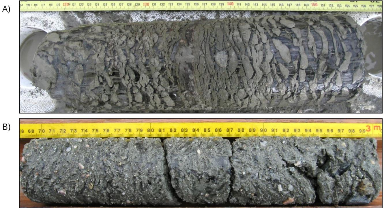
**Figure 8** Ice-rich permafrost cores extracted from A) the post-glacial marine silty clay at the valley bottom and B) the silty till deposits covering the slopes and plateaus.
