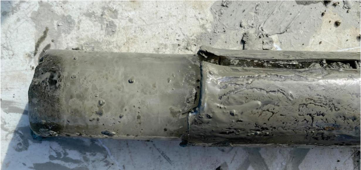
Bh J: 1-12.2 m Enlarge picture of the pure ice core encountered between 11.60 -12.20 m.
