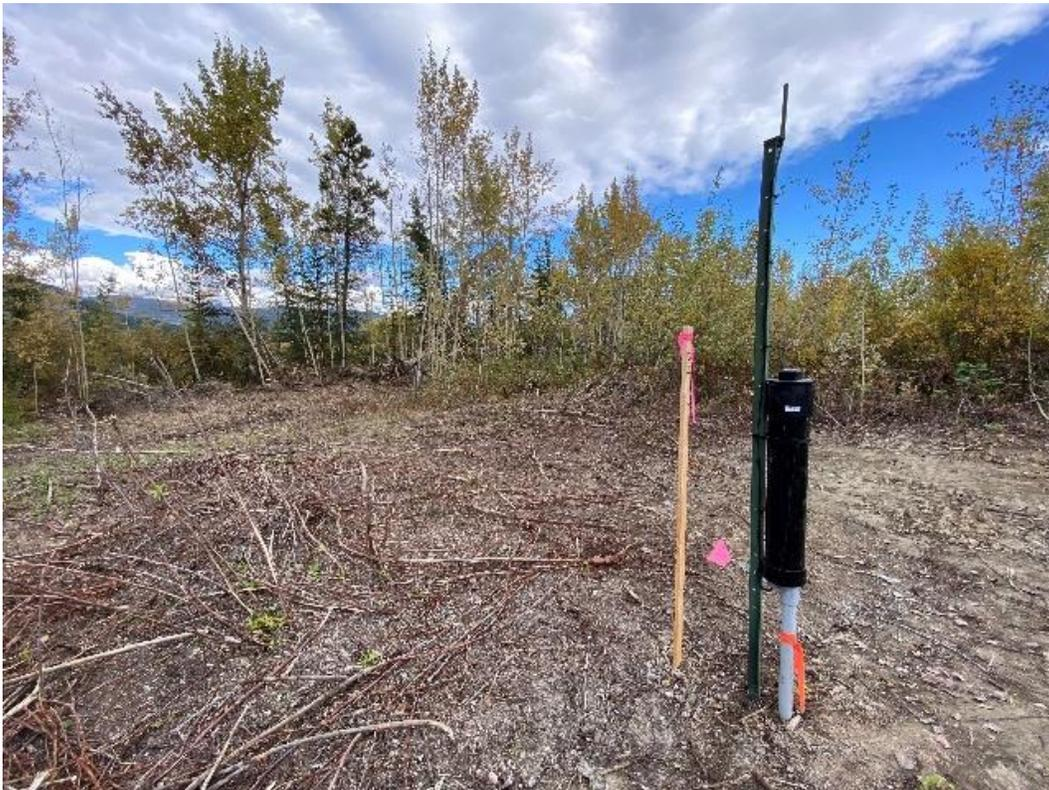
**Figure 116** LogR Systems ULOGC32 LoRa+ logger inside ABS casing at Borehole A. The antenna connected to the logger allows communication with the Gateway using long range spectrum modulation.
