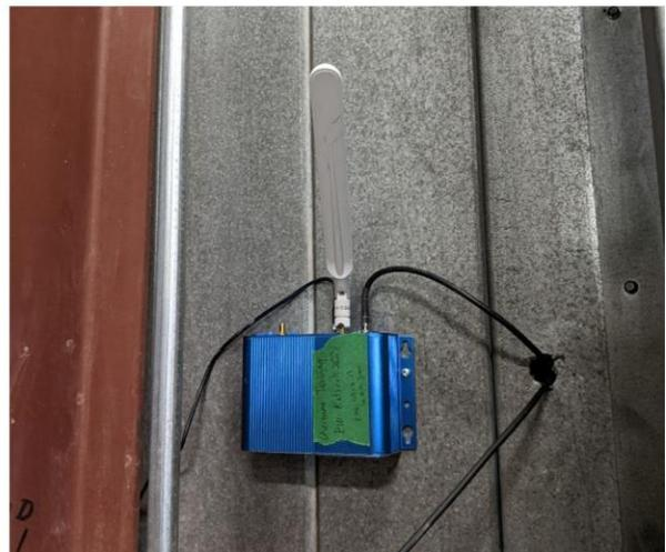
**Figure 20** A) Tasiujaq runway LoRaWAN network configuration with the proposed gateway location and end-nodes locations (ground temperature monitoring stations). B) Gateway external antenna fixed to the north-west wall at a height of about 3 m. C) Gateway located inside the airport garage.
