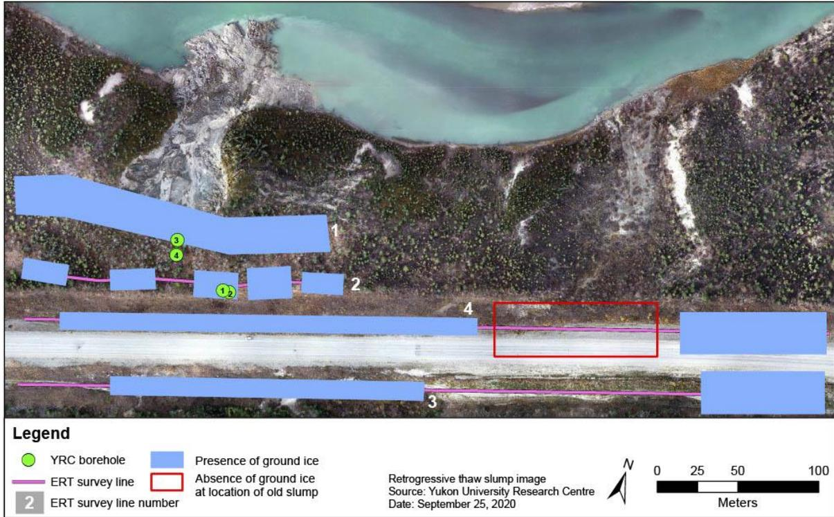
**Figure 95** Approximate position of ground ice based on ERT profiles.
