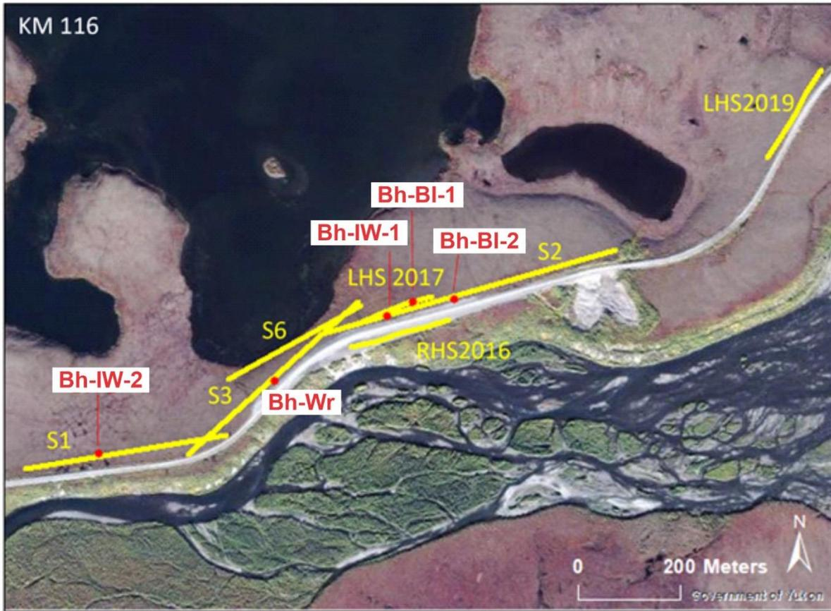
**Figure 43** Locations of the boreholes and ERT surveys at Chapman Lake section (km 116).
