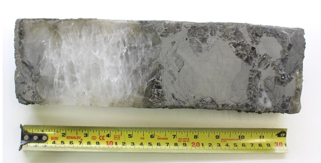
**Figure 15. Ice rich permafrost showing thick layered (left) and suspended (right) cryostructures in a core from WH\_1456\_BH1 at 657 centimeter depth.**
