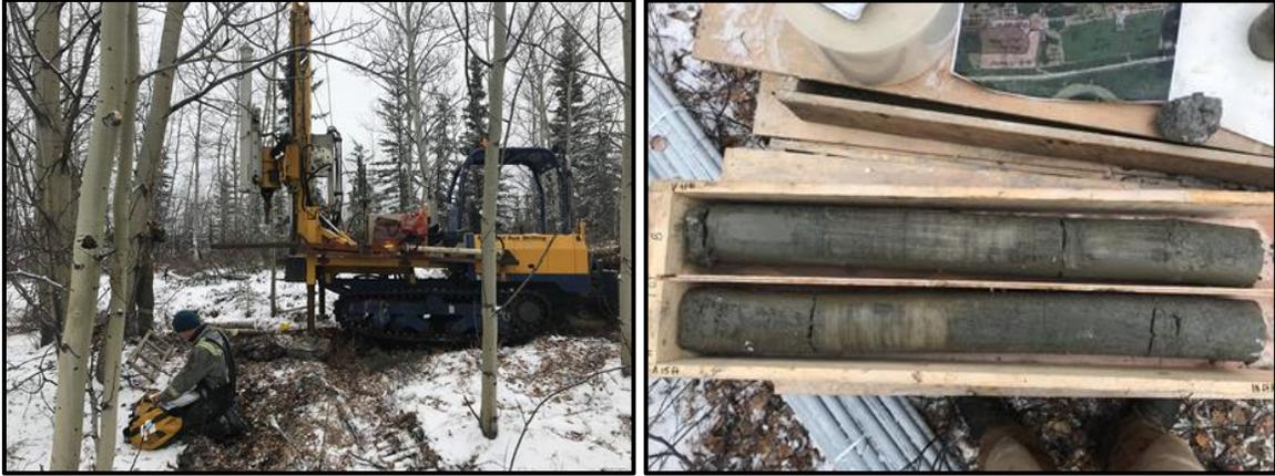
Figure 6. Midnight Sun Drilling CRREL drill rig and permafrost cores (WH\_1456\_BH1)
