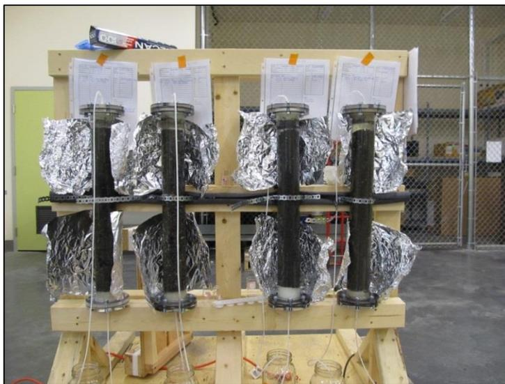
**Figure 2: Bench-scale bioreactors**
