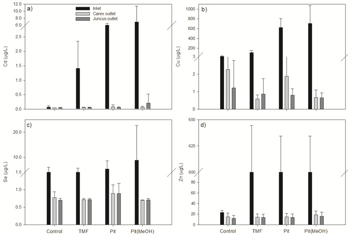
**Figure 2: Cd (a), Cu (b), Se (c) and Zn (d) concentrations in CWs with *C. aquatilis* (Carex) and *J. balticus* (Juncus) fed with Control, TMF, Pit or Pit(MeOH) waters (Note the broken Y-axis which accommodate inlet concentrations)**
