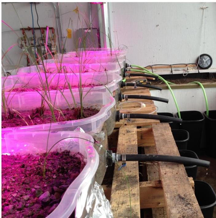
**Figure 1: Laboratory-scale CWs**
