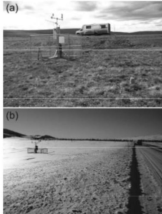
Figure 4. Site 2 shown (a) in summer and (b) in winter to illustrate the accumulation of snow beside the road embankment.
