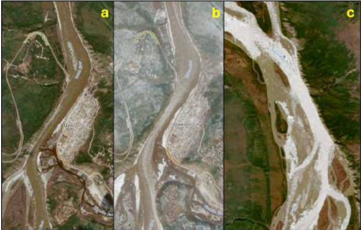
Figure 3.2.1. Sample of three Sentinel 2 satellite images of the Yukon River with different spring breakup ice run intensities. a. Light ice run with dispersed ice floes at Dawson, b. Moderate ice run with a relatively high ice concentration at Dawson, c. Full concentration ice run near the Sixty Mile River upstream of Dawson. Credit: European Union – Copernicus Sentinel Data 2026.
