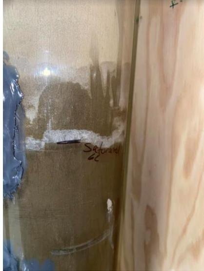
**Figure 15.** Ice pocket between the saturation point and dry inert material.
