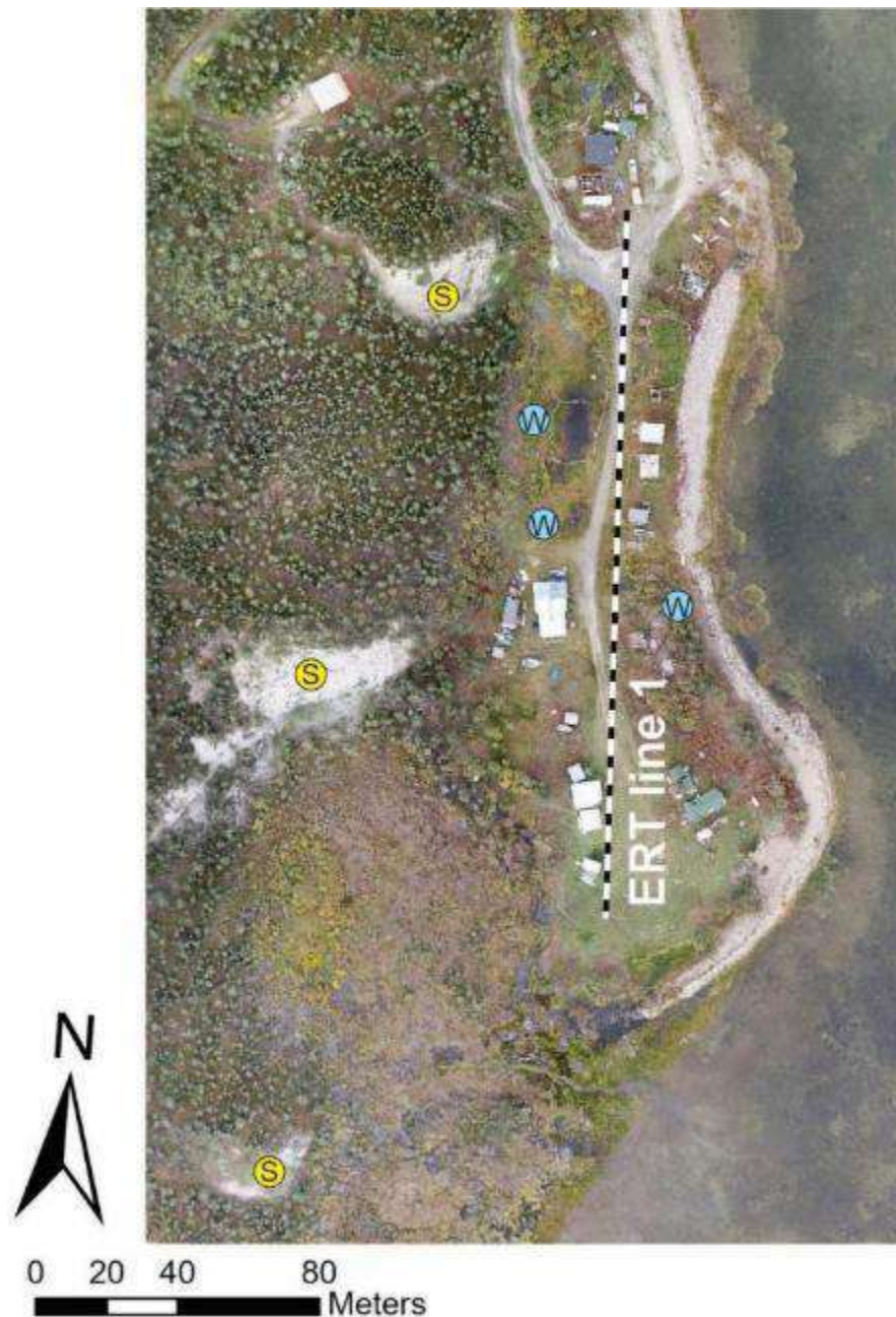
FIGURE 11 AERIAL IMAGE OF ÄSHÈYI ON THE LAKE SHORE, WHERE SLOPE INSTABILITY (YELLOW S SYMBOL) AND SUBSIDENCE (BLUE W SYMBOL) ARE SEEN.
