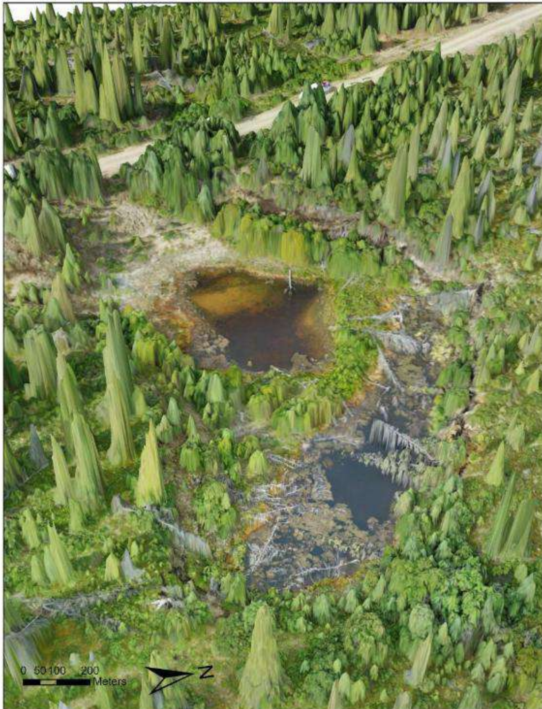
FIGURE 61 THREE-DIMENSIONAL REPRESENTATION OF THERMOKARST POND , FROM DRONE AERIAL IMAGERY. STEEP EDGES (RIDGES) ARE FORMING, AND TREES ARE COLLAPSING WHILE THE POND IS GROWING.
