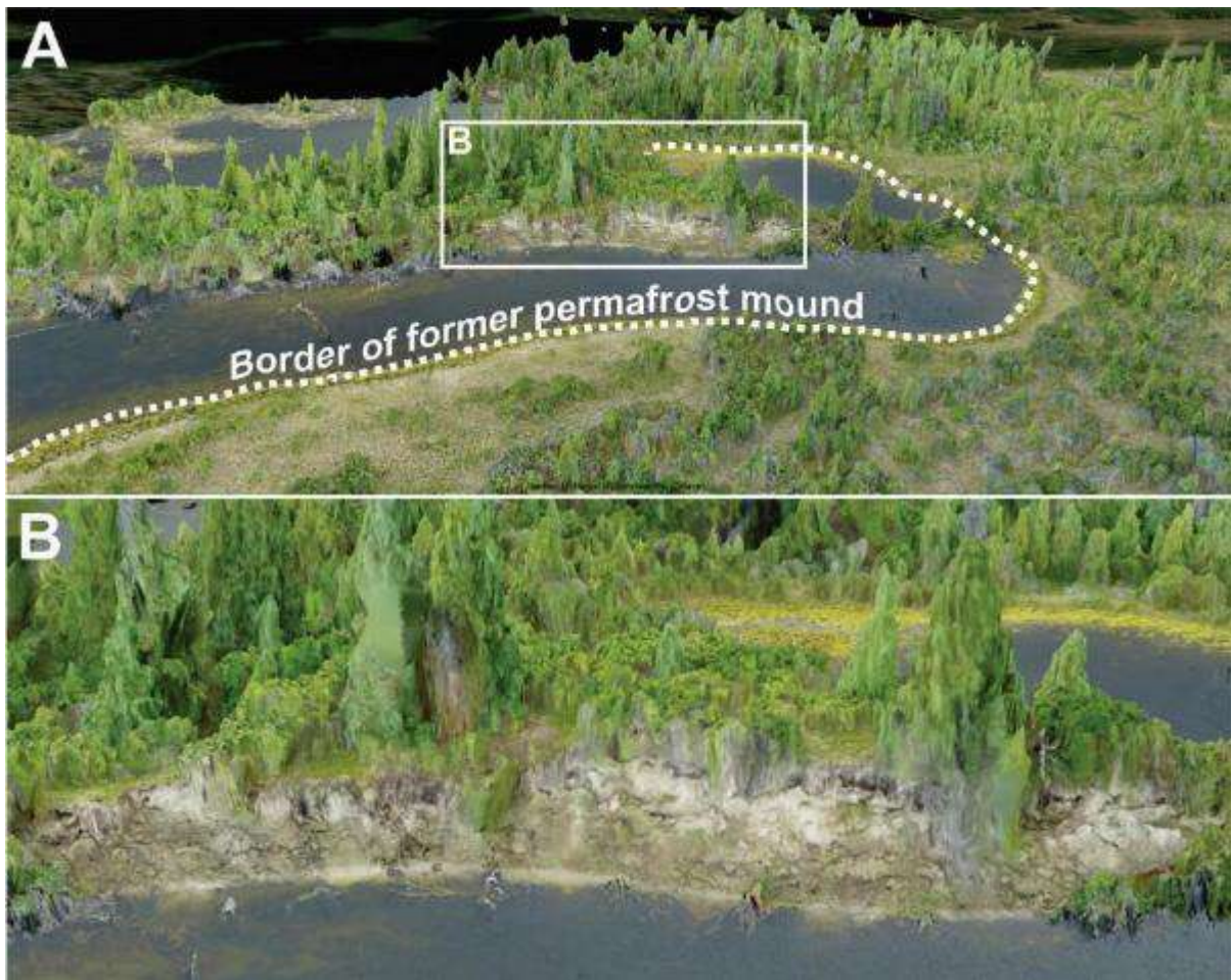
FIGURE 54 THREE-DIMENSIONAL VIEWS OF A DEGRADING PERMAFROST MOUND IN THE WETLAND OF PERMAFROST VALLEY. A- PERMAFROST MOUND SURROUNDED BY A THERMOKARST LAKE RESULTING FROM THE THAW OF THE MOUND; B- COLLAPSING EDGE OF THE DEGRADING PERMAFROST MOUND.
