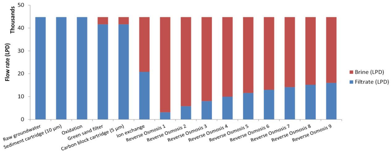
Figure 6: Water recovery observed with treatment train A, which consisted in 1 Sediment cartridge stage, 1 Green sand stage, 1 Carbon block cartridge stage, 1 Ion exchange stage, and 9 Reverse Osmosis stages.
