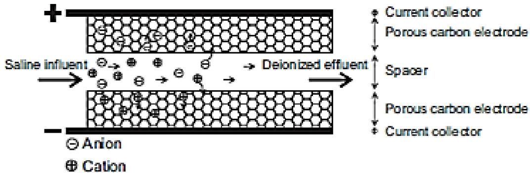
Figure 3: Capacitive Deionization principle.
