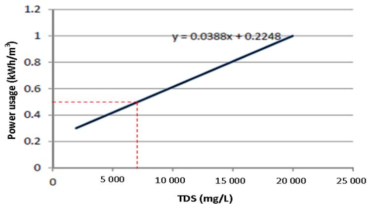
Figure 11: Power usage of one *Prestige* full-scale unit. The dashed lines represent the power usage (0.50 kWh/m<sup>3</sup>) at a feed water content of 7 200 mg/L TDS. (adapted from EWP, 2014a)
