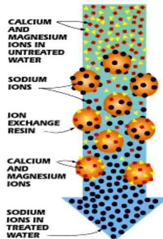
Figure 2: Ion exchange principle.
