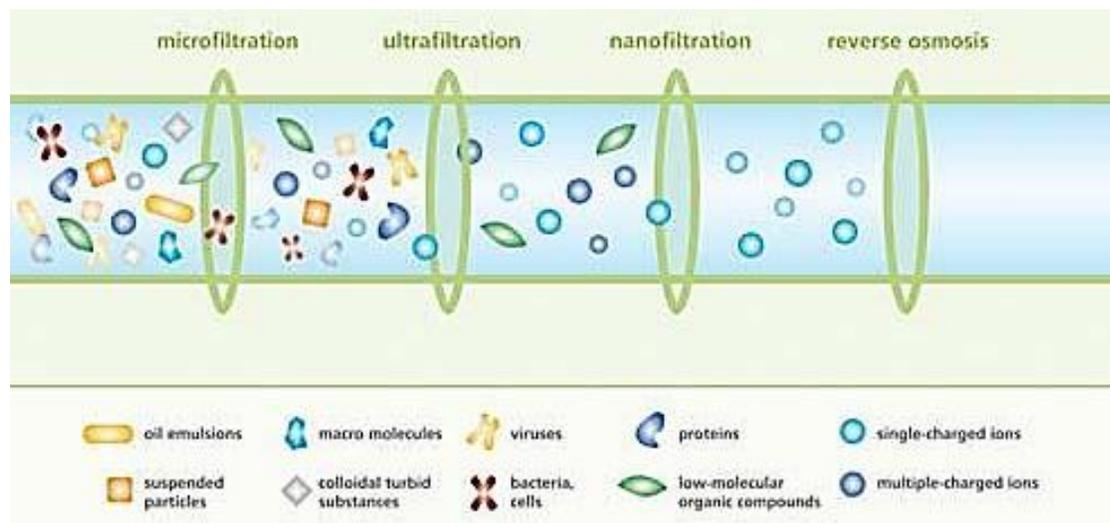
Figure 1: Particle removal capacity of filtration processes in relation to particle size.
