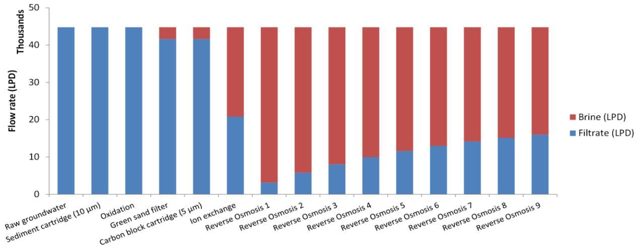
Figure 6). The green sand filter would produce 43 111 LPD of filtrate, and reject 1 333 LPD of brine. The ion exchanger would produce 21 555.5 LPD of filtrate and reject 21 555.5 LPD of brine. The reverse osmosis system would produce 16 598 LPD of filtrate and reject 4 958 LPD of brine.
