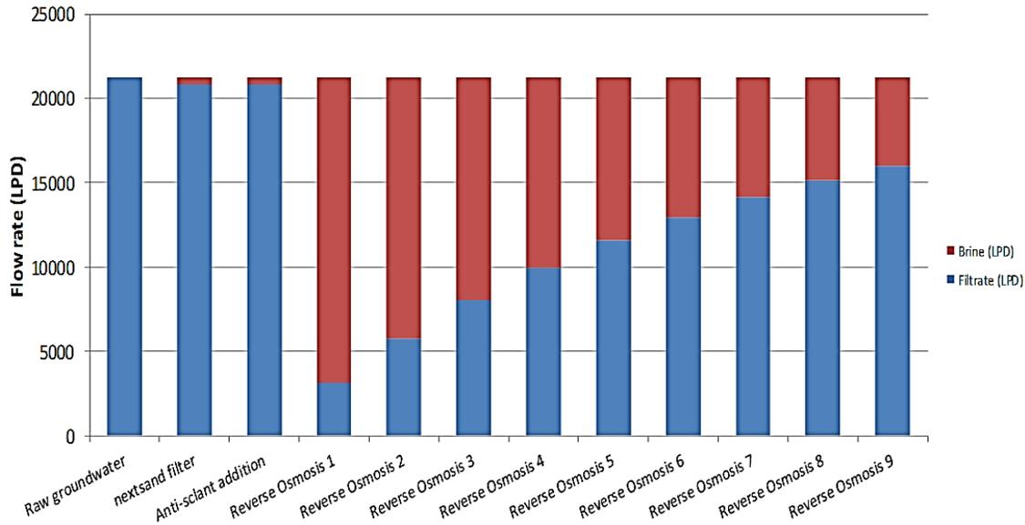
Figure 13: Water recovery observed with treatment train C, which consisted in 1 *nextsand*™ stage, and 9 Reverse osmosis stages.
