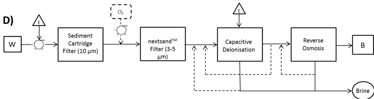
Figure 15: Recommended composite treatment train for provision of drinking water from brackish groundwater available at Northern Cross' base camp in Eagle Plains (Yukon, Canada).
