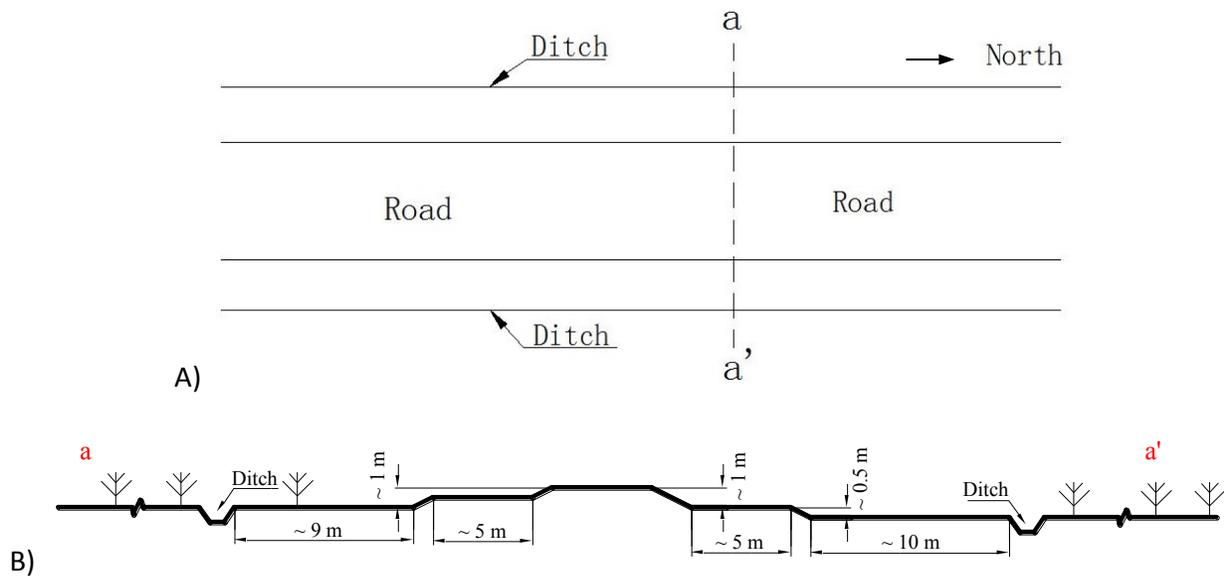
**Figure 4.3.7. Schematic illustration of the Enger Creek adaptation site for A) Localisation of proposed embankment cross section and transverse profile; and B) a-a' embankment cross section at km 1863.5.**
