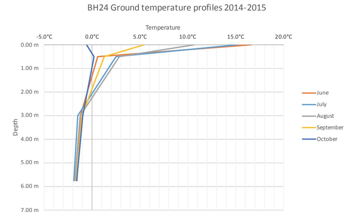
Figure 4.1.6. Ground temperature recorded in BH24 from June to October 2015.
