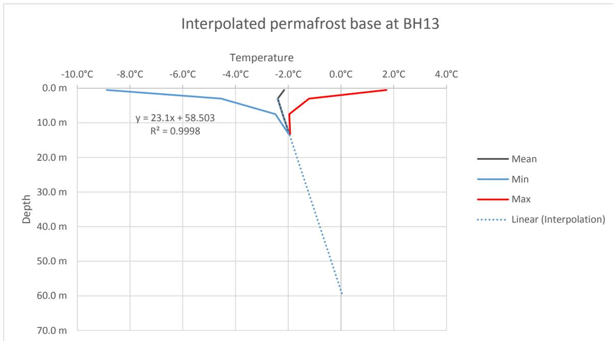
Figure 4.4.8. Interpolation of the permafrost base at BH13.
