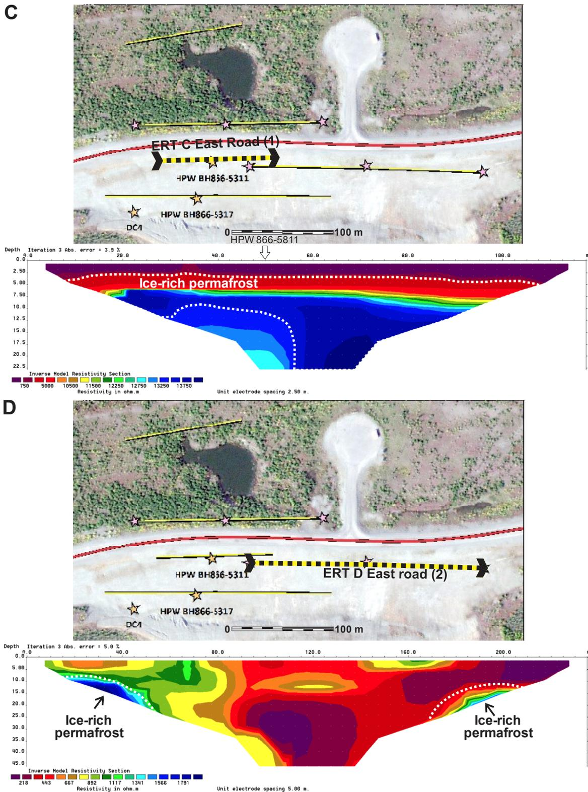
Figure 4.2.6 (cont.). ERT Surveys performed at Dry Creek rest area site for C) East of the road (North); and D) East of the Road (South).
