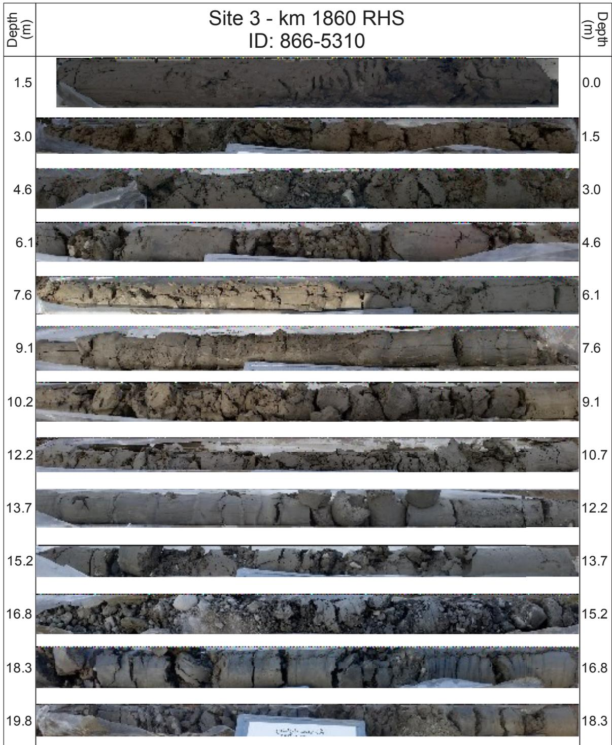
Figure 4.3.4. Cores collected from borehole HPW 866-5310
