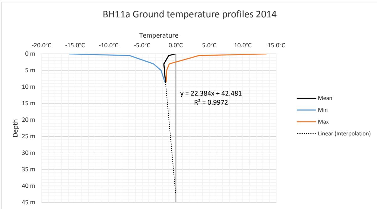
Figure 4.5.9. Interpolation of the permafrost base at BH11a
