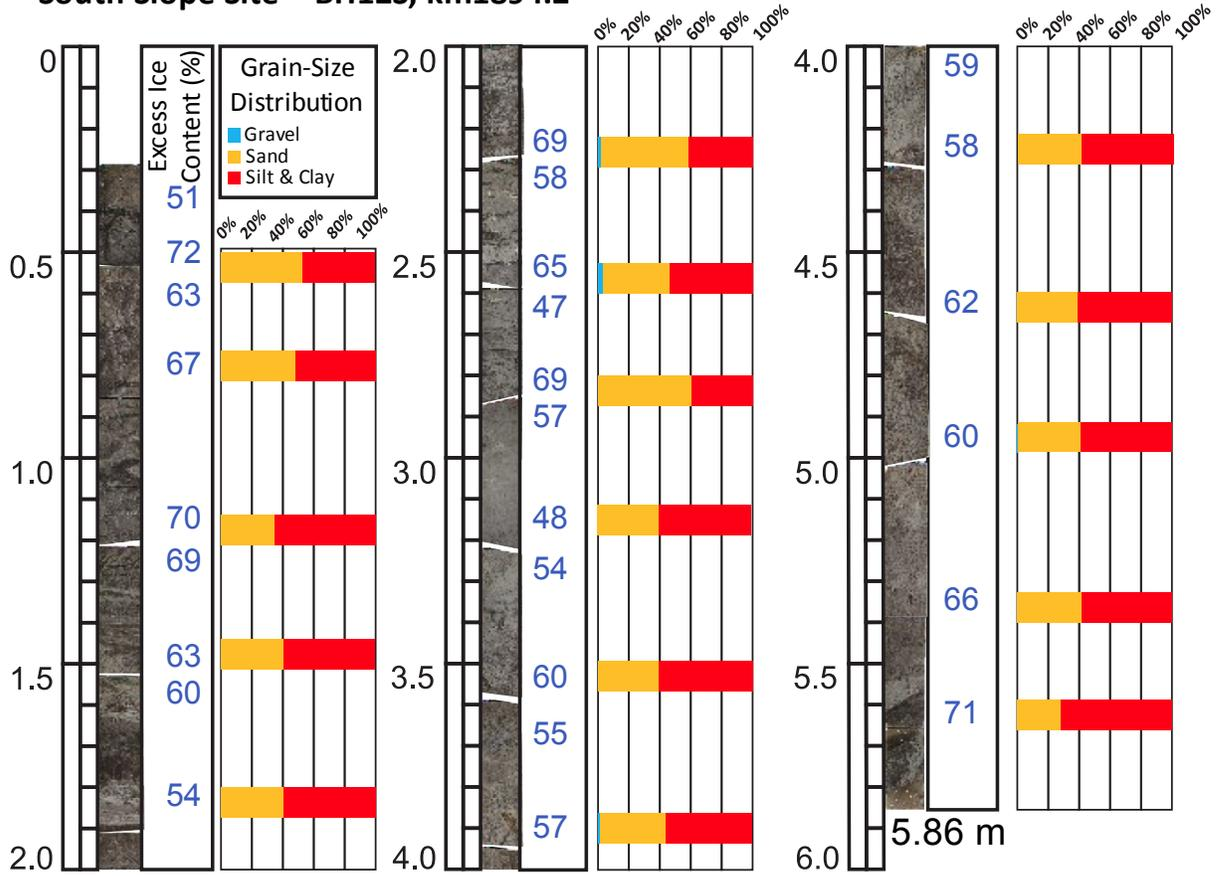
Figure 4.6.3. Log of borehole BH12S.
