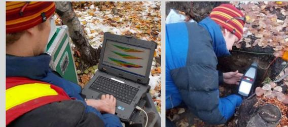
Figure 8. Measuring Electrical Resistivity and pXRF of KdV6 Sediments
