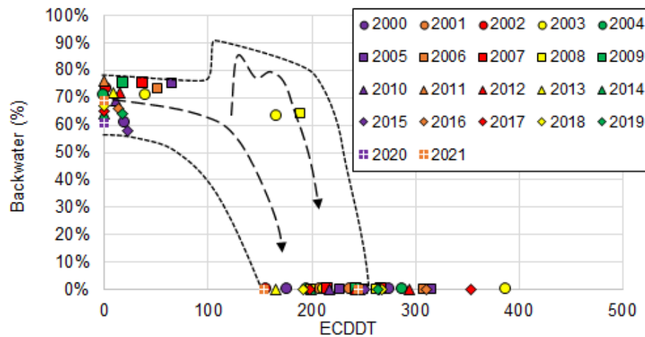
FIGURE 5.3. CALCULATED ICE-INDUCED BACKWATER – EFFECTIVE CUMULATED DEGREE-DAYS OF THAW (ECDDT) RELATIONS FROM 2000 TO 2021 FOR THE LIAR RIVER AT UPPER LIARD, AND INTERPRETED ENVELOPES (SMALL DASH LINES) AS WELL AS TYPICAL TRENDS (LONG DASH LINES, THE HIGHEST LINE PRESENTING THE ICE JAM SCENARIO).
